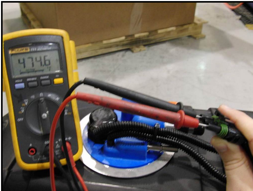
Use an ohm meter to get a reading from the connector leads and correlate the reading to a temperature
