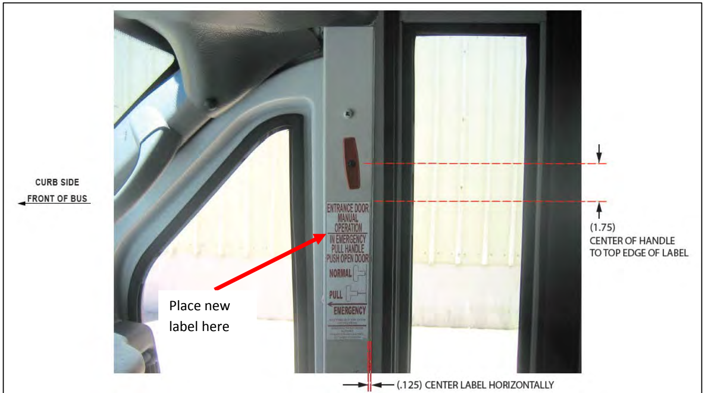
Figure 2, New Label Location
