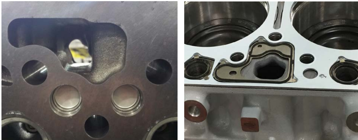
Figure1. New DD13 Cylinder Head (Left) and New DD13 Cylinder Head Gasket (Right)
