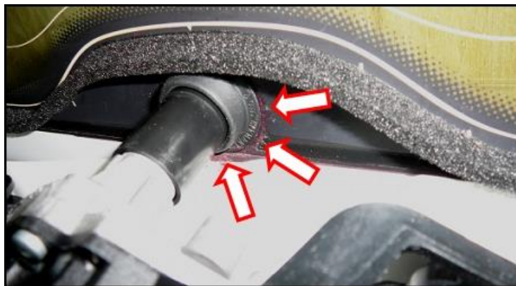
Figure 3 – Seal for the rear wiper shaft leaks
