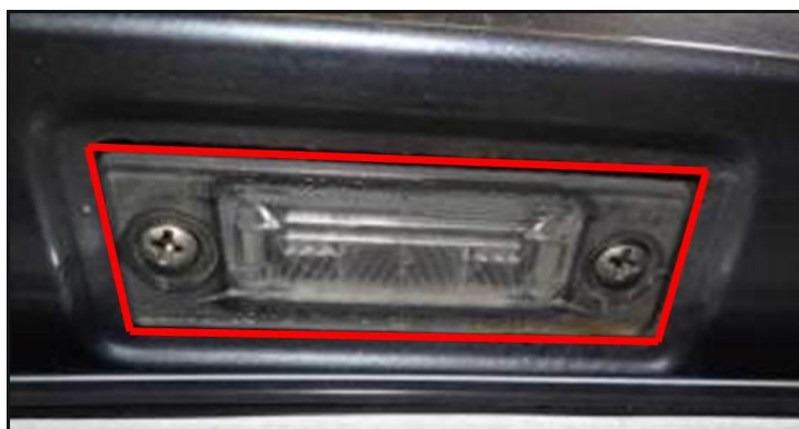
Figure 1 – Corrosion on and around the license plate light (Screw fastened light)
