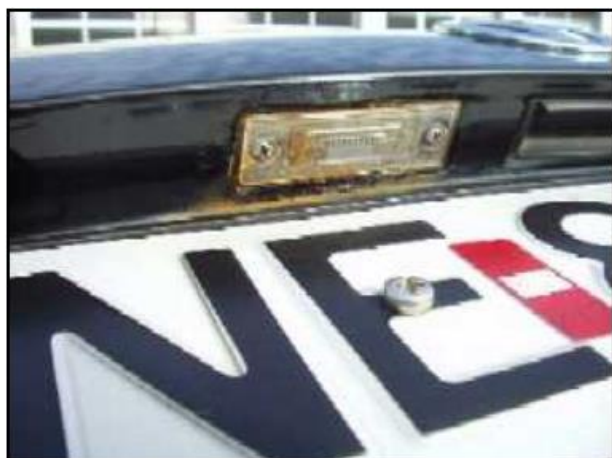
Figure 1 – Corrosion around License Plate Light
