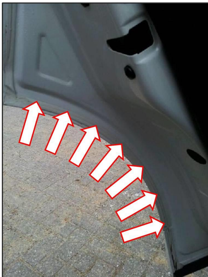
Figure 1) Arrows show the area affected by corrosion
