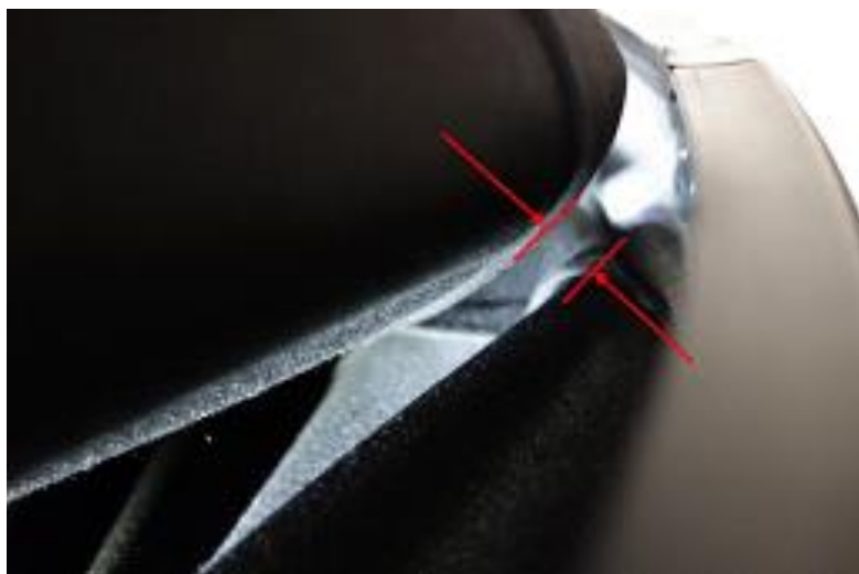
Figure 4: Ensure a 3 mm gap exists between the folds of the convertible top cover when stored (both sides).
