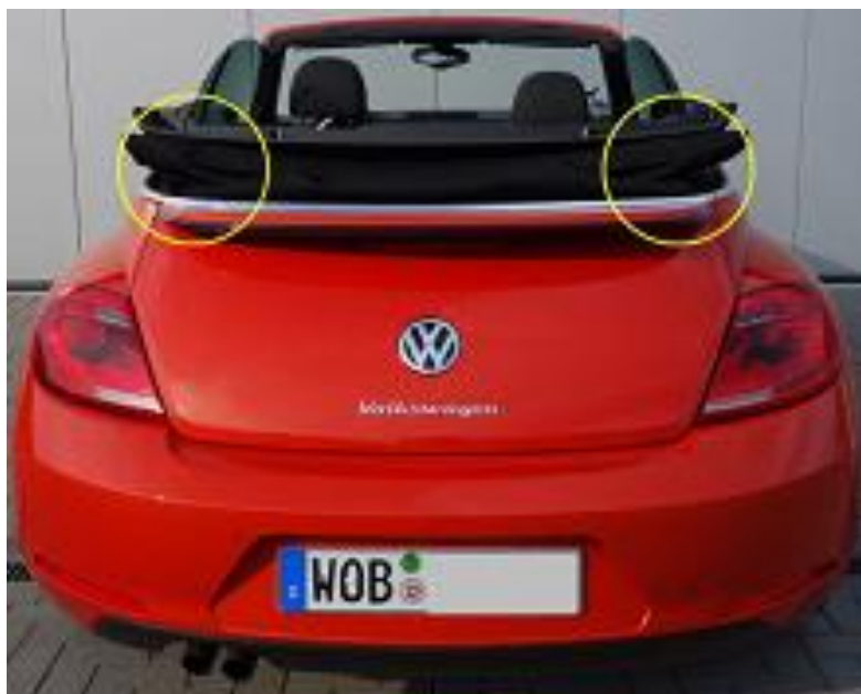
Figure 2: Overview of convertible top cover when stored.
