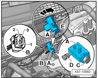
Remove the Air Quality Sensor –G238– (with the humidity sensor in fresh air intake duct – G6570) <A> by rotating 90° and remove it from the fresh air intake <E>.
