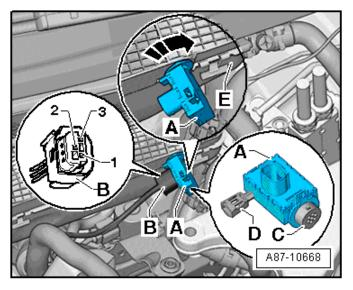
Reinstall the Air Quality Sensor -G238- (with • the humidity sensor in fresh air intake duct -G6570) <A> in the fresh air intake <E> by rotating 90°.
