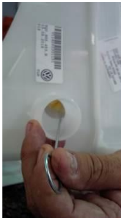
Figure 4. Cleaning the sensor probes.
