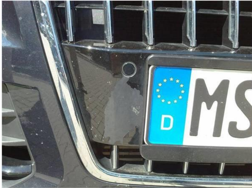
Figure 1. Example of flaked-off paint.
