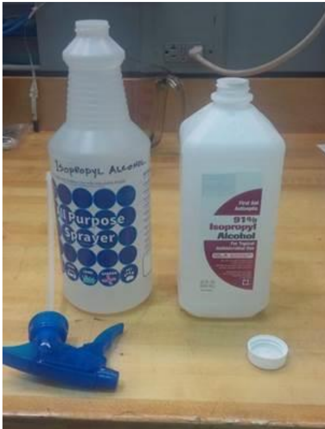
Figure 2. Filling a general purpose spray bottle with Isopropyl alcohol to aid in the contact surface preparation.
