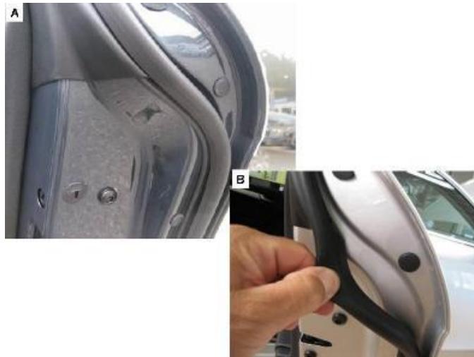
Figure 3. The door seal pressed to the door (A), and detached again (B).
