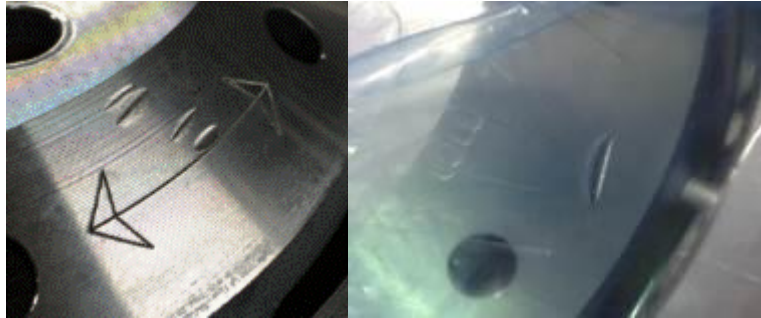
Figure 1: Example of disc brake with impact marks that should NOT be installed.
