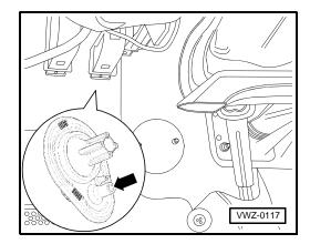
Connect the 5 cables to the larger of the two plug connectors on the engine control unit in accordance with the corresponding table. Tick off each work step in the "Completed" column of the table. Cross out tables which are not required.
