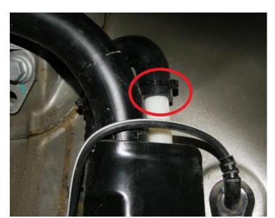
Install the assembly onto the open end of the vent pipe and secure with a Tie strap as shown.
