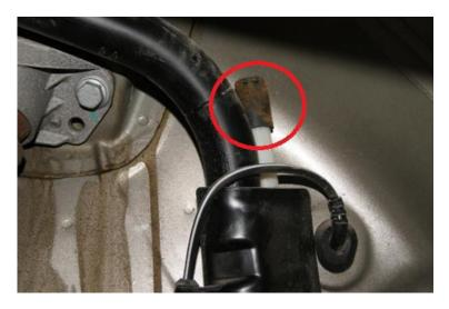
Remove the right rear wheel, wheel well liner and the rubber vent cap from the tank vent pipe. Inspect the vent line near the bottom of the filler neck for water/ice buildup. Use a vacuum device to clean.
