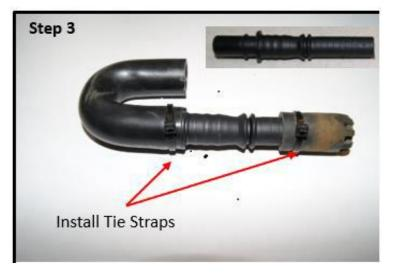
Install the vent cap and U shaped rubber hose onto the previously cut tube from step 2.
