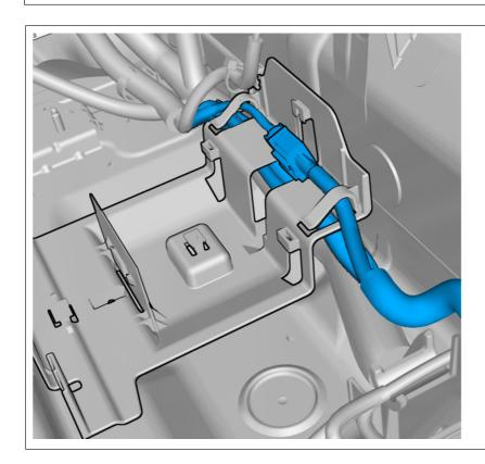
Route the cable harness to the existing cable harness.
