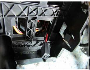
**Step 10**: Remove the red and black wire from starter relay connector and install in the new starter relay harness connector.
