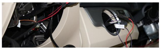
**Step 3:** Remove 8mm nut and add the brown ground wire to the steering column ground location.
