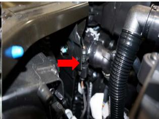
**Step 11:** Check to see if hood latch micro switch is already installed. If so skip this step, If not remove hood latch and install the micro switch into the hood latch.
