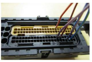
**Step 9:** : Insert the Red/Black wire in location K45 (Remove and insolate wire already in this location if applicable), Insert the Red/White wire in location K88, Insert the Blue/Red wire in location K25, insert the Blue/Green wire in location K26, insert the Violet/White wire in location K44.
