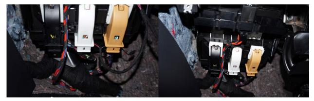
**Step 7:** Insert the red/blue wire into location B14, Insert the black wire into location C31, Insert the red/white wire into location C34, Remove the wire from location C30 and insert into the supplied connector position 1 and connect to the violet/white wire connector.
