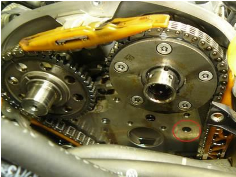
Figure 6. Test point of oil duct (red circle) to non-return valve in cylinder head
