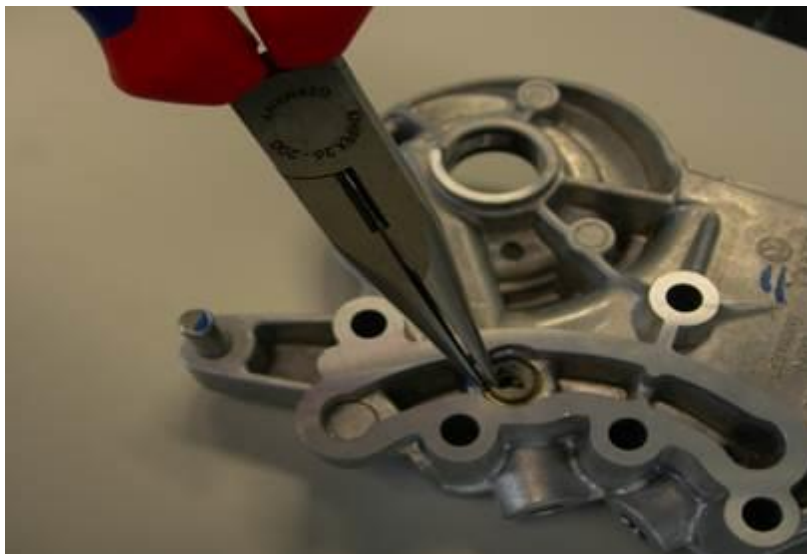
Figure 3. Remove the strainer.
