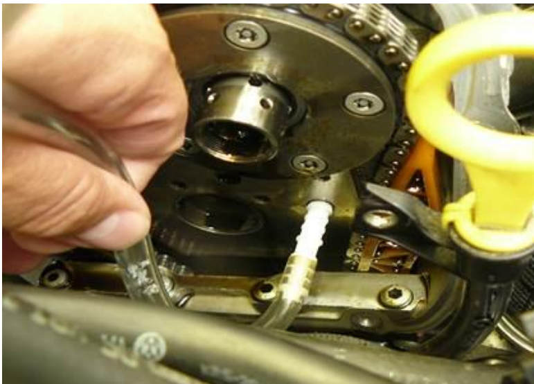
Figure 7. Press pressure line with adapter of VAS 6213 firmly into oil duct hole
