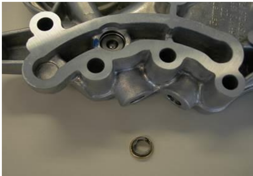
Figure 4. Camshaft bearing bracket with metal non-return valve (without strainer)
