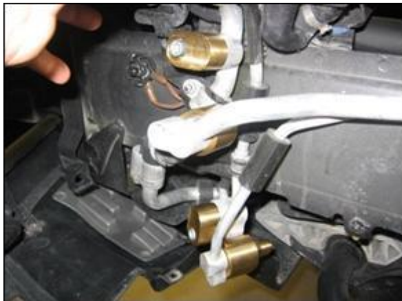
Figure 8. The location of the connections inside the left front wheelhouse on a Touareg with four zone climate control.
