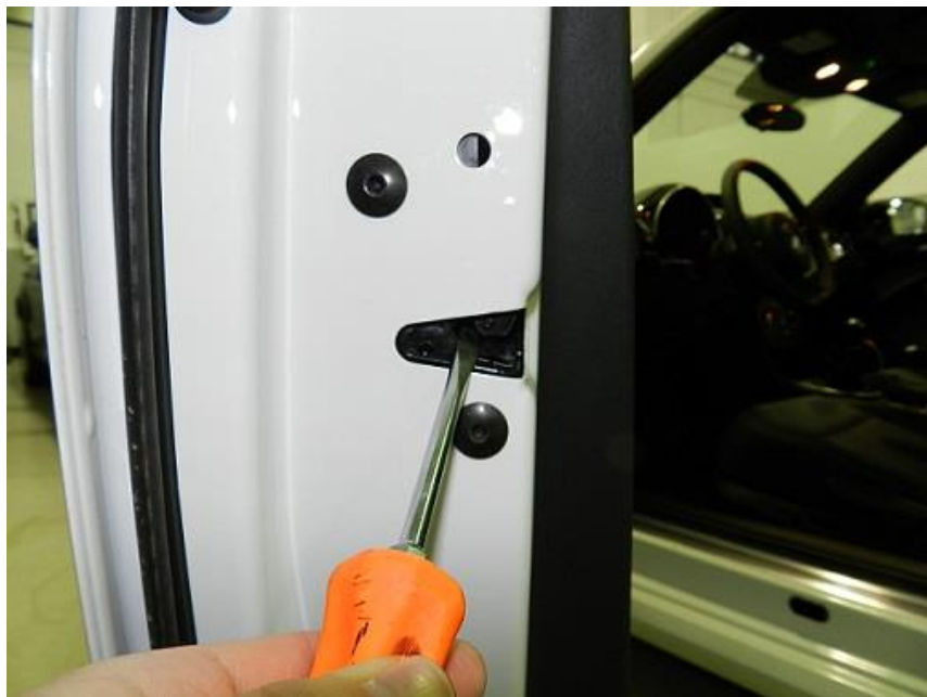
Figure 4 (Manually close the catch in the door latch)
