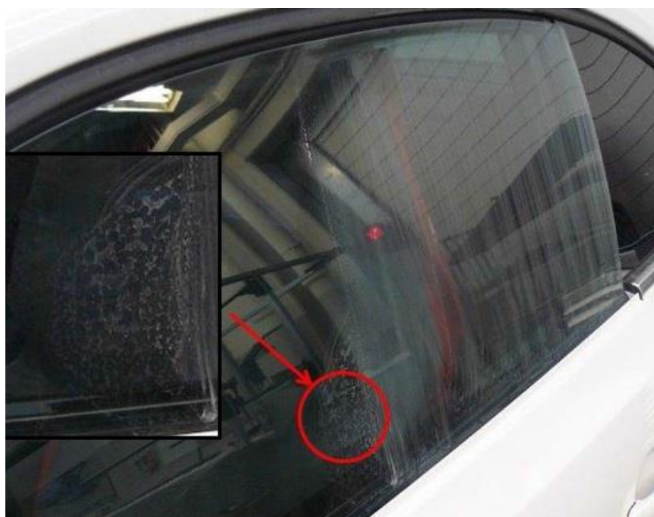
Figure 6 (insufficient treatment of window with cleaning cloth)
