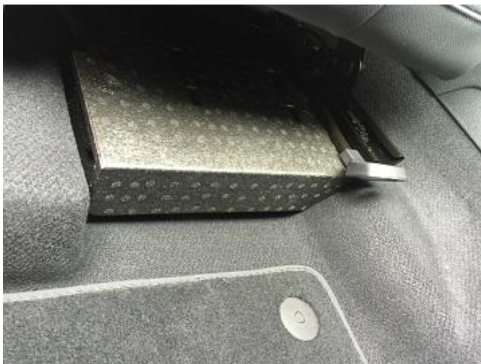
Figure 1: Car-Net module housing loose
