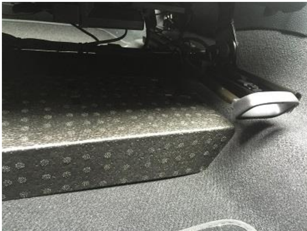
Figure 5: Car-Net module housing properly installed.
