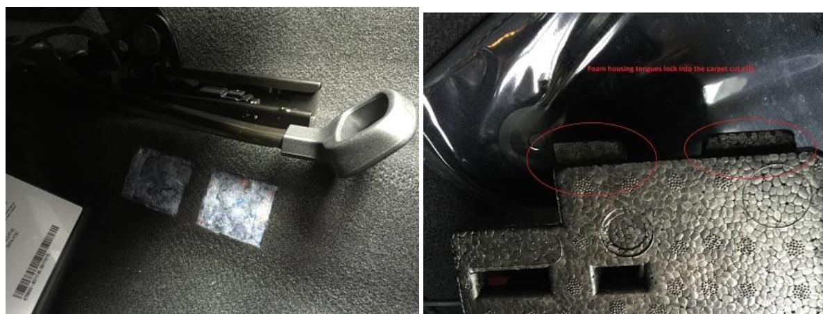
Figures 3 and 4: Carpet cut-outs removed and locking tabs on housing
