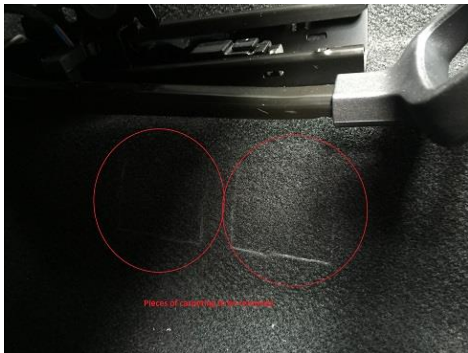
Figure 2: Pre-perforated carpet cut-outs not removed
