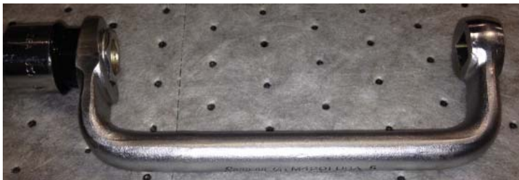
OFFSET 7/8 WRENCH (CYLINDER HEAD WRENCH), SNAP-ON PART NUMBER M4201
