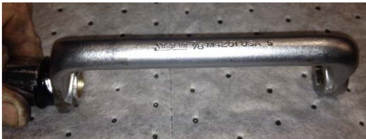
OFFSET 7/8 WRENCH (CYLINDER HEAD WRENCH), SNAP-ON PART NUMBER M4201
