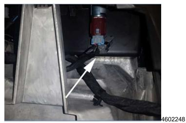
2. Remove the USB harness from the power outlet receptacle harness.
