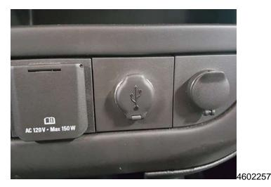
4. Install the USB receptacle to the instrument panel.
