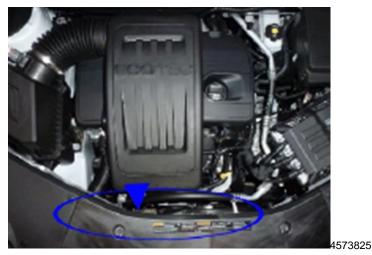
2. Locate the black painted engine cradle centered directly below the radiator and engine.
