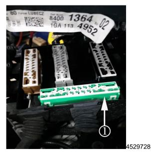
26. Install the forward lamp harness connector (1) into the engine wiring harness junction block bracket.
