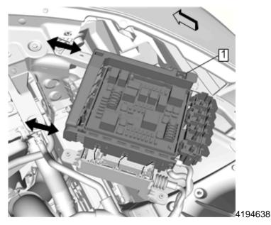
6. Slide the locking bar forward to release the engine wiring harness junction block (1) from the engine wiring harness junction block bracket.
