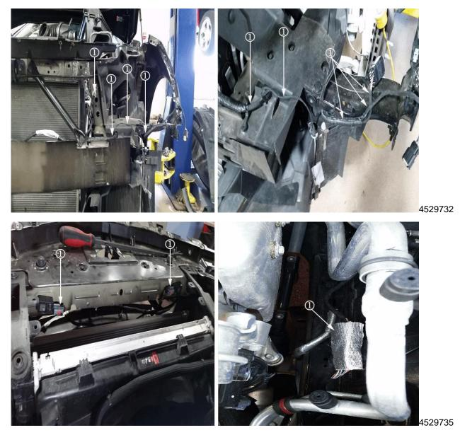
**Caution:** Note the routing of the forward lamp harness prior to removing it. Harness chafing and/or damage could occur if the forward lamp harness is routed improperly when reinstalling.
