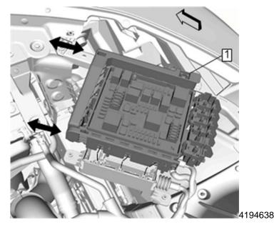
27. Install the engine wiring harness junction block (1) to the bracket. Slide the locking bar rearward to lock the engine wiring harness junction block to the bracket.
