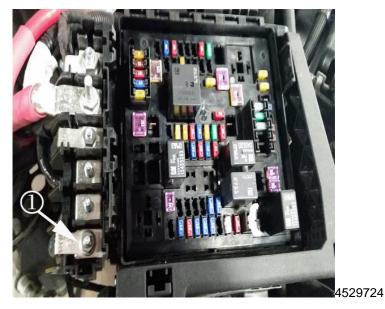
5. Disconnect the forward lamp wiring harness cable (1).
