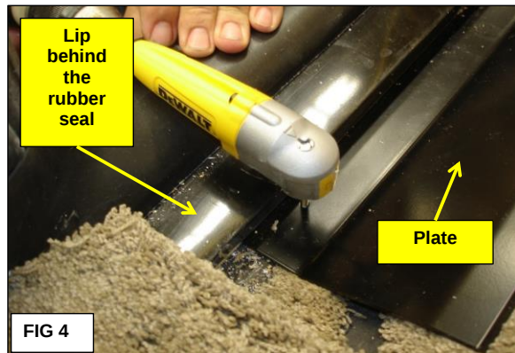
Fig 4: Place the plate behind the seal, and under the lip of the slideout. (Picture taken before slideout is installed).
