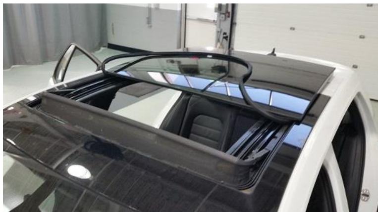
Figure 6 (Inner sunroof seal draped over sunroof glass)
