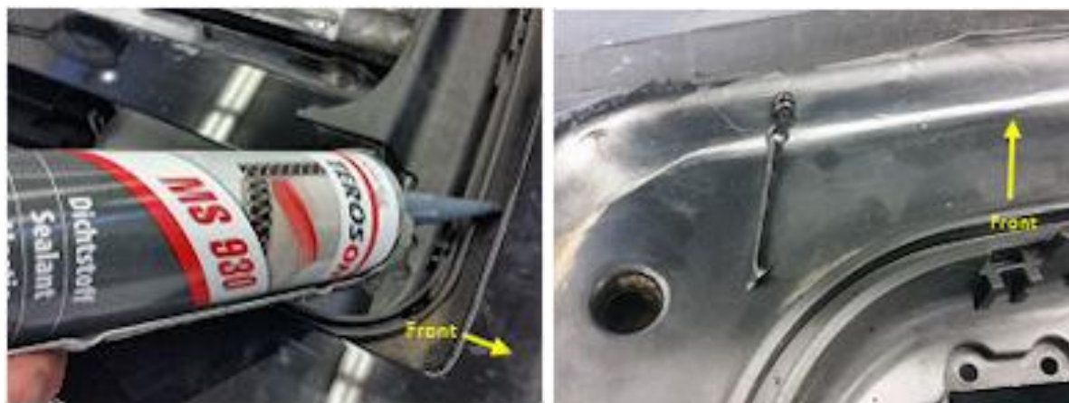
Figures 10 and 11 (Sealant application)
