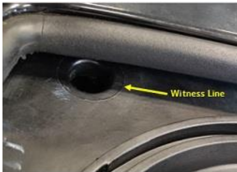
Figure 15 Drain hole and witness line.
