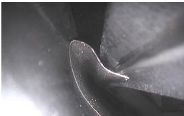
Figure 27 Foil folded and not adhered underneath trim panel
