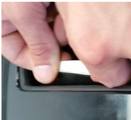
Figure 21 Use a pivoting motion to work foil underneath trim panel in position 4.
