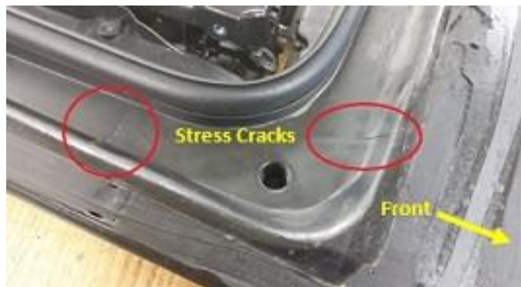
Figure 2 (Examples of stress cracks in water channel)
