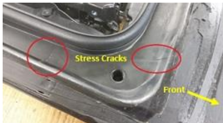
Figure 2 (Examples of stress cracks in water channel)
