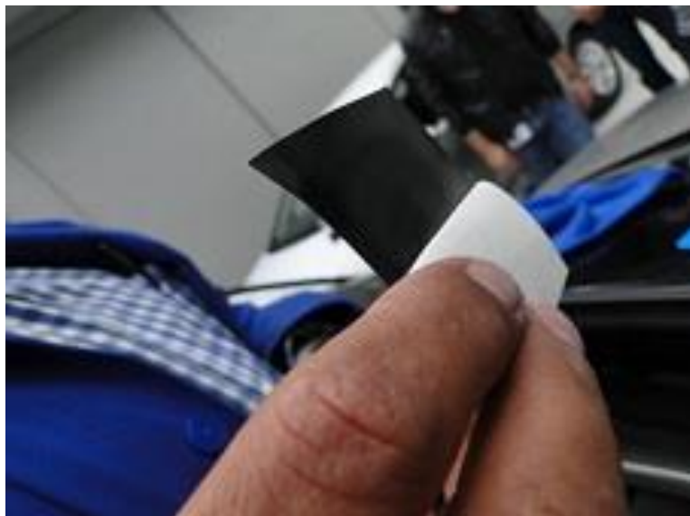
Figure 16 Peel half of backing tape off foil and fold in half to use to hold the foil as it is applied.
