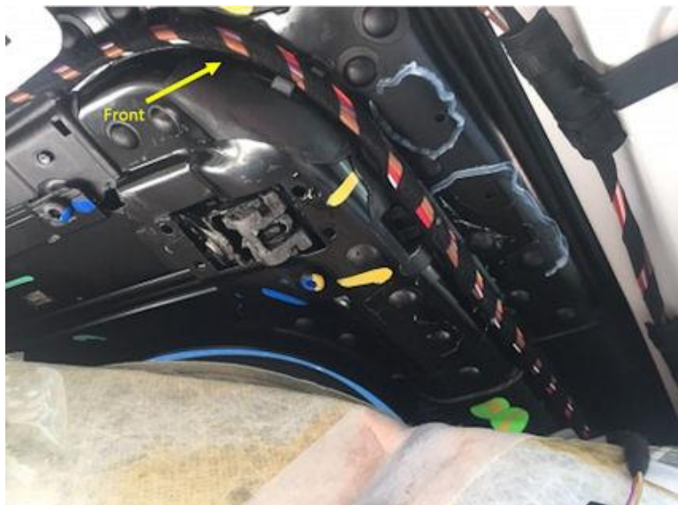
Figure 1 (Water leaking through corner of water channel)
