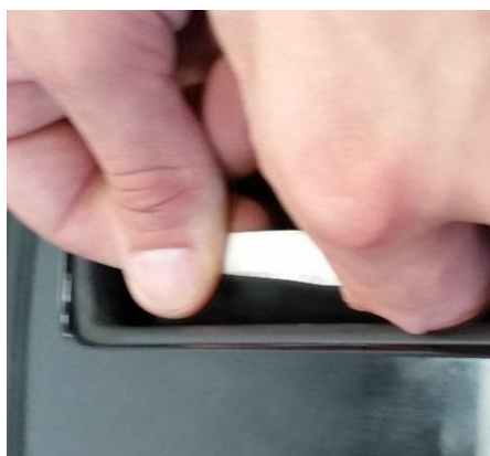
Figure 21 Use a pivoting motion to work foil underneath trim panel in position 4.
