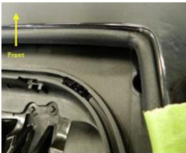
Figure 20 Foil position 3 incorrectly applied covering witness line around drain.
