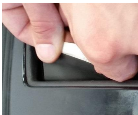
Figure 21 Use a pivoting motion to work foil underneath trim panel in position 4.
