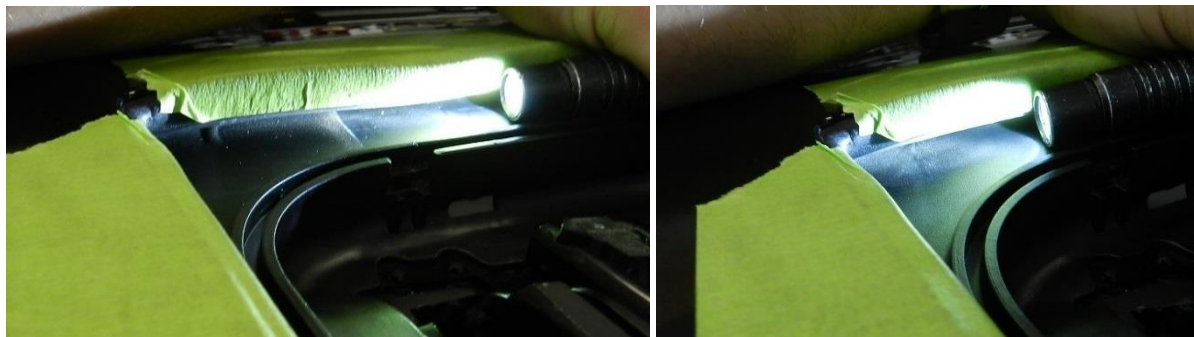
Figure 25 and 26 use a flashlight to help identify any air bubbles in the foils and use the squeegee to work out any defects.
