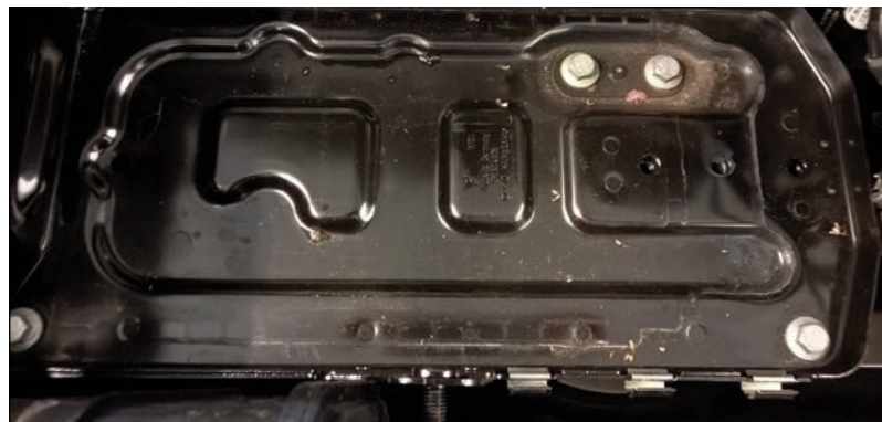
9P1804825 Battery tray for 70Ah (I195), 80Ah (I196), 95Ah (I200), 40Ah Li-ion (I192) without additional bracket
