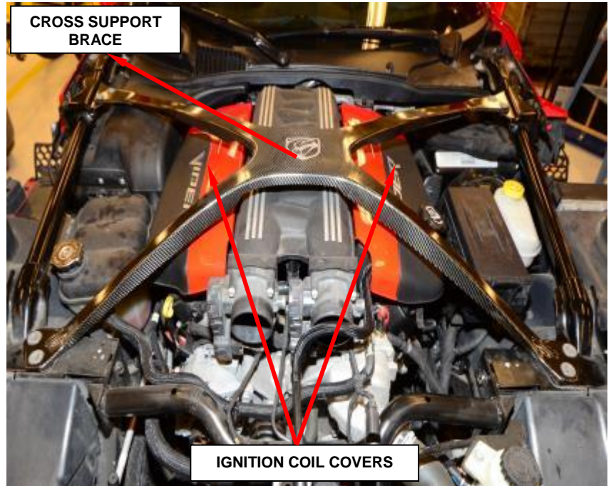
Figure 14 – Cross Support Brace
