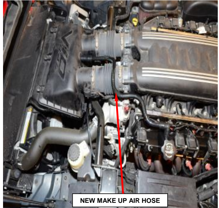
Figure 7 – New Make Up Air Hose
