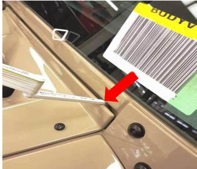
Fig. 8 Feeler Gauge Between Windshield And Cowl
