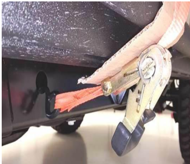
Fig. 10 Strap Hooked In Frame Hole
