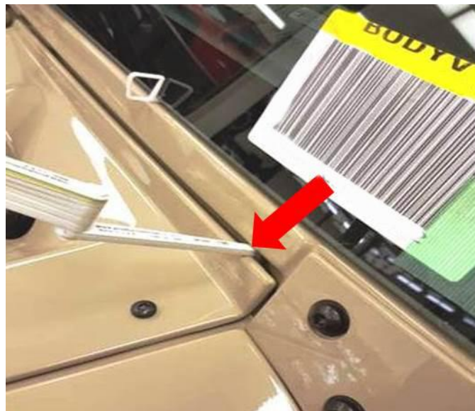
Fig. 13 Feeler Gauge Between Windshield And Cowl
