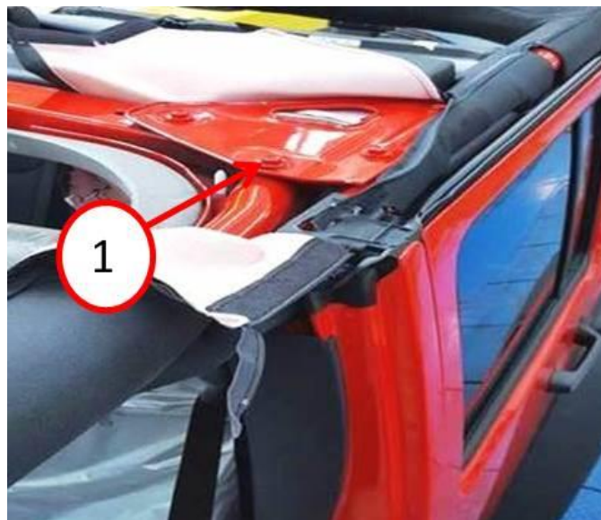
Fig. 2 Top Of The Side bar Bolt
