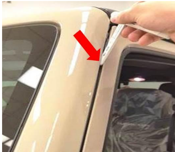
Fig. 12 Feeler Gauge Between Door And Windshield Frame
