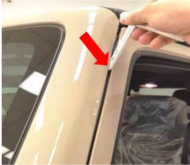
Fig. 5 Feeler Gauge Between Door And Windshield Frame
