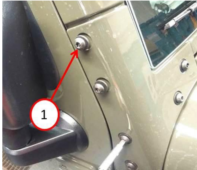
Fig. 3 Loosening Six Gusset Bolts
