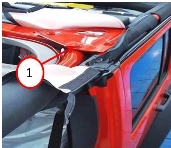
Fig. 7 Top Of The Side bar Bolt
