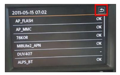
If the screen freezes on the following screen, hold down the power button on the radio for 10 seconds to reboot the J794. The software update should start where it left off.
