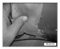
This condition may be due to the foam pad on the inner fender pressing against the upper edge of the fender, which chafes through the paint in the affected area.
