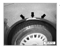
Corrosion at front fender -arrows-, as shown.
