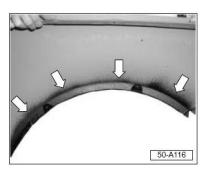
Apply the 3M<sup>™</sup> Underseal Rubberized Undercoating, Part No: 08883, around the entire inner fender wheel arch flange while ensuring 100 percent coverage.
