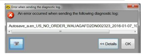
**A.** These logs were saved when the ODIS Service **Connection Type** is/was set to **CPN**. Diagnostic logs created with connection type CPN **cannot be transmitted** to GFF Paperless.
