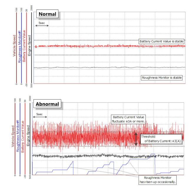
The abnormalities shown above for the Roughness Monitor and Battery Current Value are a result of resonance originating in the alternator pulley assembly. Although a DTC P0300 can also be set, there is not an actual misfire of the engine.
