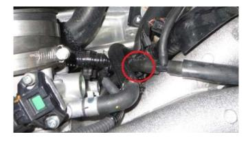
**Step 29:** Pull on the vacuum hose to remove it from the connection on the intake manifold. \*\*Note the routing of this vacuum hose as it will be used for installation of the new hose in **Step 31**.
