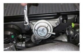
**Step 25:** Remove the 2 bolts securing the PCV pipe to the intercooler. Loosen the 2 hose clamps securing the intercooler to the turbocharger and intercooler to throttle body.
