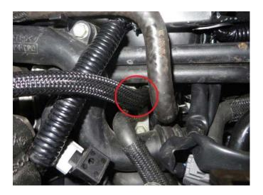
**Step 21:** Reinstall intercooler, tighten the hose clamp to 26.4 inch-pounds and torque the 2 bolts on the turbocharger to 11.8 foot-pounds.
