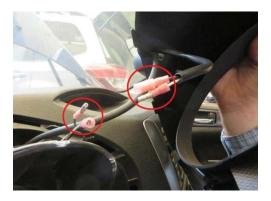
**Step 5:** Remove the vacuum hose from the elbow and pull it through the bottom of the combination meter hood. The hood can now be completely removed.
