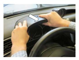
Step 4: After removing the combination meter hood, disconnect the boost gauge wiring connectors.
