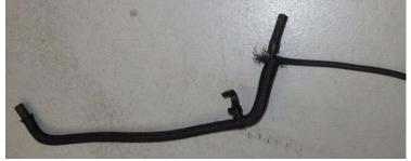
**Step 19:** Release the tab on the hose clip and remove it from the original hose. Reinstall this clip in the same position on the new hose.
