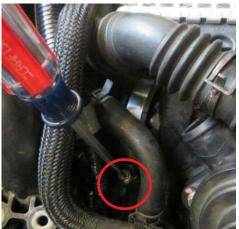
**Step 15:** Follow the vacuum hose coming from recirculation valve and disconnect it from the port where it connects to the engine. \*\*Note the routing of this hose as it will be used for installation of the new vacuum hose in **Step 20**.
