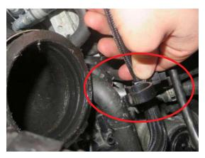
**Step 17:** Follow the boost gauge vacuum hose coming from the t-fitting to the bulkhead. Remove the bulkhead grommet and gently feed the hose through firewall into the engine compartment while ensuring nothing gets caught by the hose on the inside of the vehicle. Install the new bulkhead plug.
