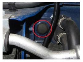
**Step 18:** Cut any wire ties used to secure the boost gauge vacuum hose then remove all hoses connected to the t-fitting.
