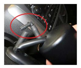
**Step 6:** Remove the 2 screws securing the combination meter to the instrument panel. **CAREFULLY** remove the combination meter enough to access the wiring harness connector. Disconnect it, remove the meter and set aside in a safe place.
