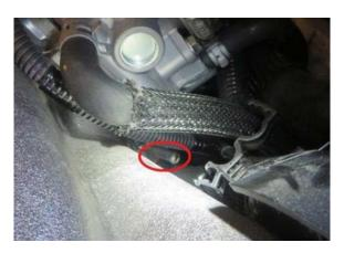
**Step 30:** Follow the boost gauge vacuum hose coming from the t-fitting to the bulkhead. Remove the bulkhead grommet and gently feed the hose through firewall into the engine compartment while ensuring nothing gets caught by the hose on the inside of the vehicle. After removing the old vacuum hose assembly, install the new bulkhead plug.
