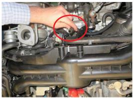
**Step 16:** Remove the hose clip from the existing hose as shown below.
