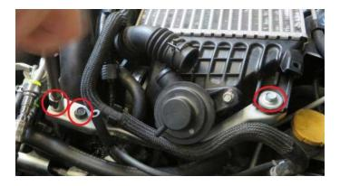
**Step 14:** Remove the 2 bolts securing the intercooler to the turbocharger, loosen the hose clamp and remove the intercooler assembly.
