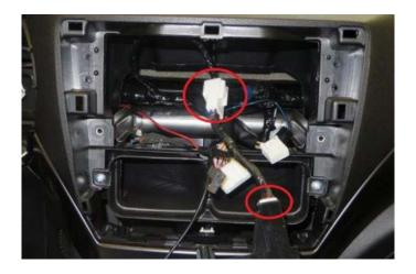
**Step 11:** Feed the boost gauge harness back through the dash. Disconnect the dimmer switch jumper from the dimmer switch, reconnect the original vehicle harness to the switch and refit the switch assembly to the instrument panel. Reinstall the instrument panel end cover trim panel.
