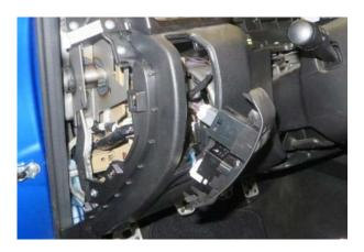
**Step 8:** Using a plastic trim tool, **CAREFULLY** remove the audio unit trim and then the 4 screws securing the unit to the instrument panel. Slide the unit out, disconnect the harness connectors and set the audio unit aside. If equipped, once the audio is removed, also remove the satellite radio receiver.
