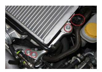
**Step 27:** After removing the bolt securing the passenger side of the intercooler, it should be free. **CAREFULLY** side the intercooler out from the 2 hose clamps previously loosened while ensuring it does not get caught on PCV piping or recirculation valve.
