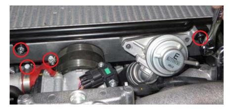
**Step 26:** Remove the hose from the clip on the intercooler. Remove the bolt securing the intercooler to the bracket and the 2 bolts securing the bracket to the engine. The bracket should now be free.
