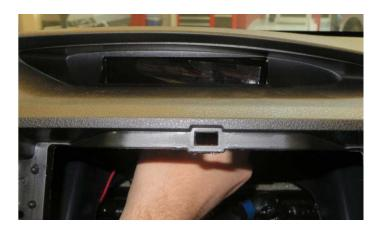
**Step 10:** Remove the boost gauge jumper harness from original clock connector and reconnect original vehicle harness back into the clock. Reinstall the clock (and satellite radio receiver).
