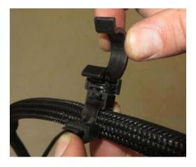
**Step 20:** Connect the new vacuum hose to the port on back side of the engine. Route the hose the same way as referenced in **Step 15**.
