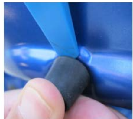
Hold Onto Stopper and Release the Opposite Side Tang
