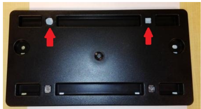
Figure 1. Damaged screw inserts
