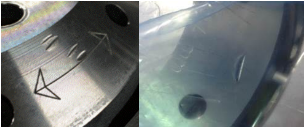
Figure 1. Example of brake disc with impact marks that should not be installed.
