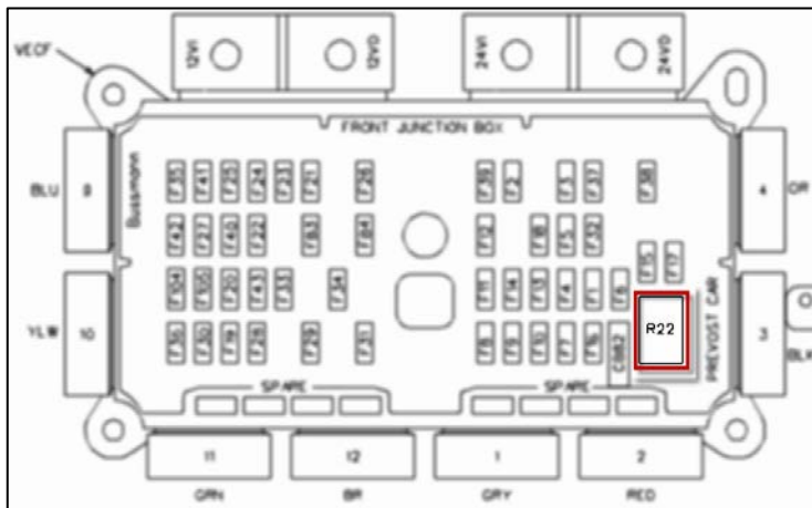
Figure 2 Typical location of R22 in VECF.
