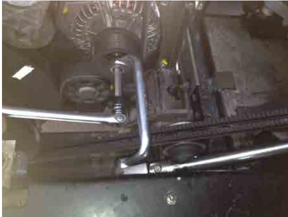
USING THE CYLINDER HEAD WRENCH WITH A RATCHET AND A FLEX SOCKET WRENCH
