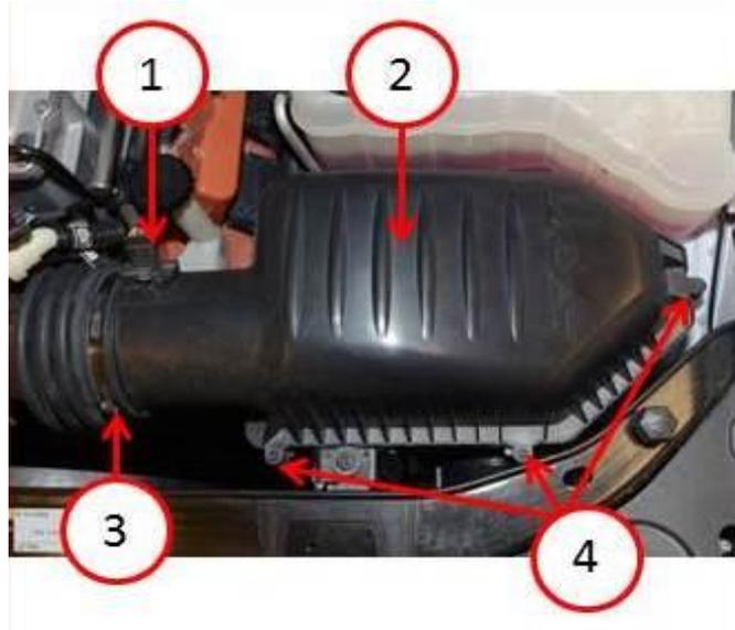
**Fig. 2 Removal Of Air Filter Housing Cover**
