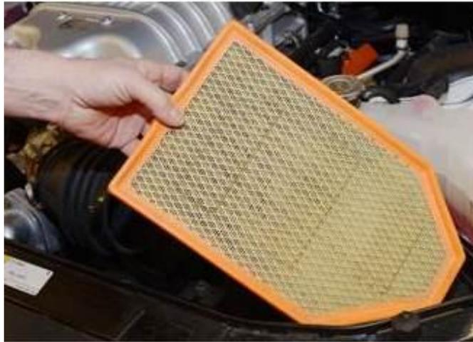
**Fig. 3 Removing Air Filter**
