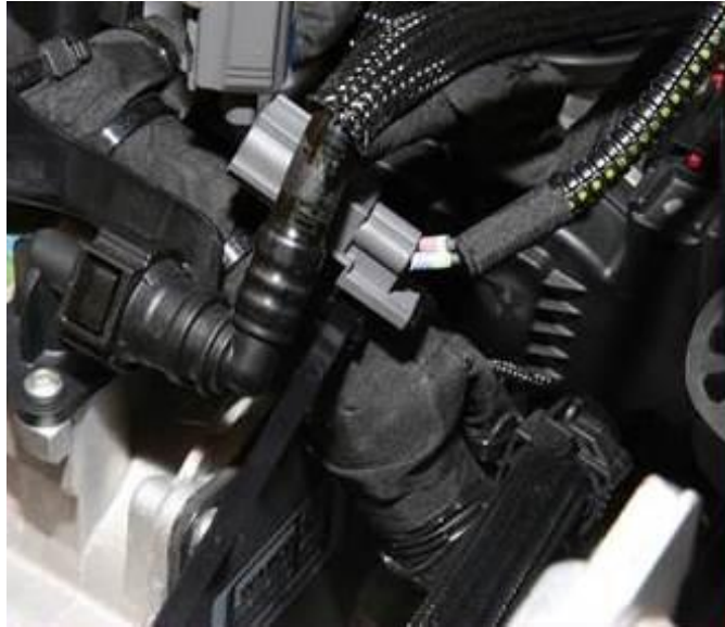
Fig. 5 Location Of Jumper Fastened To Harness
