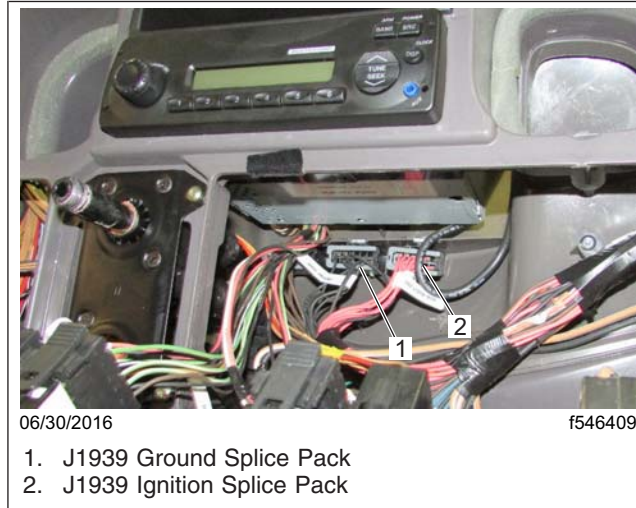
Fig. 5, J1939 Datalink Connectors
