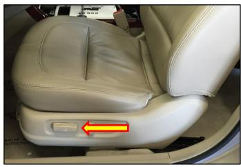
6. Remove the seat shield cover and disconnect the switch connectors.
