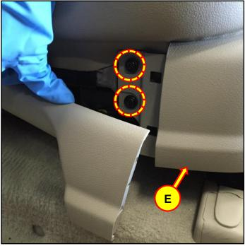
5. Move the driver seat forward to access the seat shield cover.
