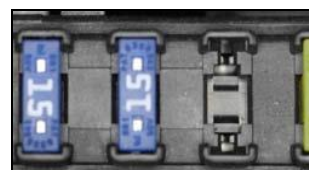
Proper Gap Between Terminals
