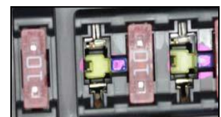
Loose Fit Between Fuse terminals
