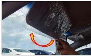
2. Position sunvisor approximately at a 45 degree angle from the headliner. Check sun visor by gently tapping the edge of the visor. Push (tap) the sunvisor with small increments until it is repositioned near the windshield. (sunvisor set up : refer to the picture)
