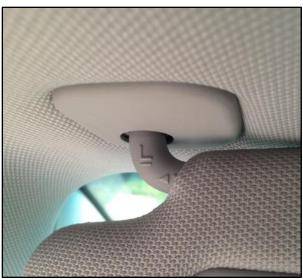
12. Verify that the visor light is working properly by operating the mirror cover. **Use labor Op-code 60CA19R1.**
