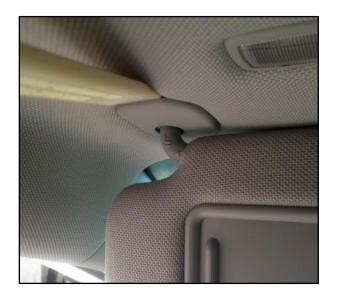
5. Remove the two bolts by using a T25 torx head screw driver.
