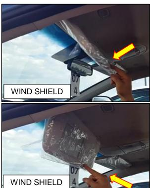
If the sunvisor maintains its position during the test, no part replacement is necessary.
