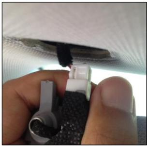
9. The groove of the sunvisor mounting cover must be assembled properly to the mounting frame. The sheet metal must sit between the grooves of the sunvisor mounting cover.
