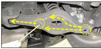
Rear Cross Member. Insert the nozzle in different directions into the rear cross member through the various openings to coat the interior with cavity wax.
