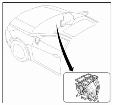
2. Remove the (2) screws from the heater core cover over the heater core tubes using a Philips screwdriver, and then remove the heater core from the assembly.
