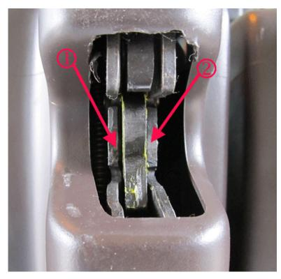
2.1 With the second row seat in the latched down position, inspect both sides of the same latch for striker to latch gapping, as shown. If gapping is present, perform the following to align the latch openings to the striker.
