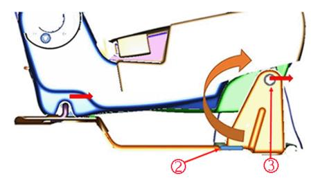
3.4 Reinstall the 60 percent seat into position. The 2.6mm washer (2), (no longer visible), at the seat-to-seat forward attachment stud (4) will be sandwiched between the 60 percent seat base and 40 percent seat base frames.
