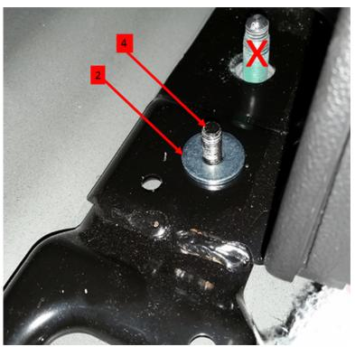
Adding the 2.6 mm washer (2), which will be sandwiched between the 40 percent seat and 60 percent seat frames, is intended to slightly tilt forward the seat riser (3), which will in turn pull the 60 percent seat inboard latch forward to help center the latch opening to the floor striker, eliminating the rattle.
