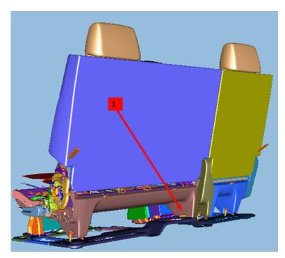
3.1 Remove the 60 percent seat (3) from the 40 percent seat (2), by removing both the seat-to-seat attachments (1) and floor attachments. Leave the 40 percent seat in position.
