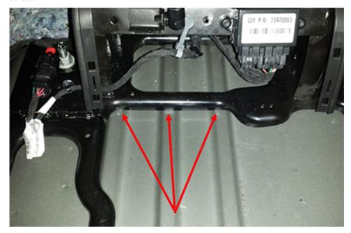
4.3 Apply Mylar tape to the floor pan to provide relief for the rattle condition, then reevaluate.
