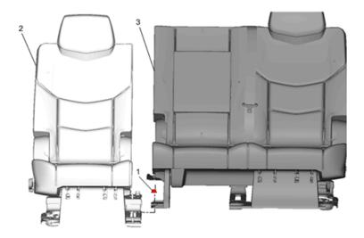
3.2 Pick up and position the 60 percent seat to allow access to the forward seat-to-seat attachment stud (4) locate on the 40 seat base, shown below.
