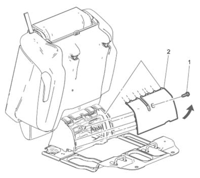
4.2 Inspect the seat base plate for contacting the ribs of the floor pan, as shown below. If contact is present paint damage may be visible at the area of contact.
