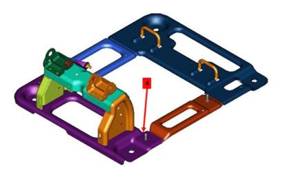
3.3 Place a 2.6 mm thick flat washer (2) over the 40 percent seat base stud (4), which is the seat-to-seat attachment, NOT the floor stud (X). This washer will be sandwiched between the 40 percent seat base and 60 percent seat base frames.
