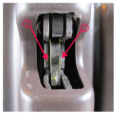
Condition 3: 60/40 Split Bench Seat: 60-percent long side bench, inboard latch (1) may not be properly aligned fore/aft in striker opening. Could cause a rattle and/or the striker to drag on the side of the latch opening not allowing the seat to flip forward or latch down easily.
