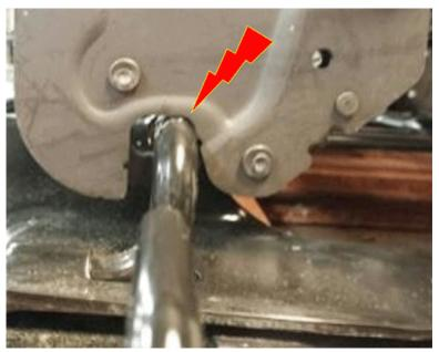
Condition 2: A seat bottom latch (inboard and/or outboard) may have an unequal latch opening side-to-side for the striker to seat into, see picture below. Opening (1) may protrude down farther than opening (2), which can cause a rattle, and which may make it difficult to secure and/or release latches.
