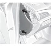
To install the end cover, insert the tabs on the back of the cover into the slots in the instrument panel at the points shown. Align the clips with the slots in the instrument panel, and press the cover into place.
