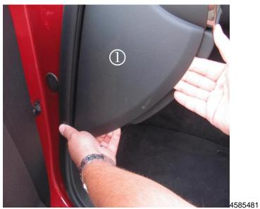
1. Remove the instrument panel outer trim cover - left side (1). Refer to *Instrument Panel Outer Trim Cover Replacement* in SI.
