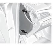
To install the end cover, insert the tabs on the back of the cover into the slots in the instrument panel at the points shown. Align the clips with the slots in the instrument panel, and press the cover into place.
