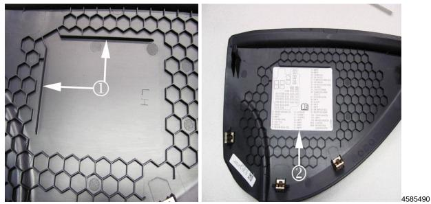
4. Using the alignment tabs (1), carefully align new label (2) to the surface. Press firmly and smooth out entire label ensuring corners are fully adhered.
