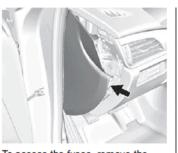
To access the fuses, remove the end panel by gently prying with a plastic tool near each clip, beginning at the point shown.
